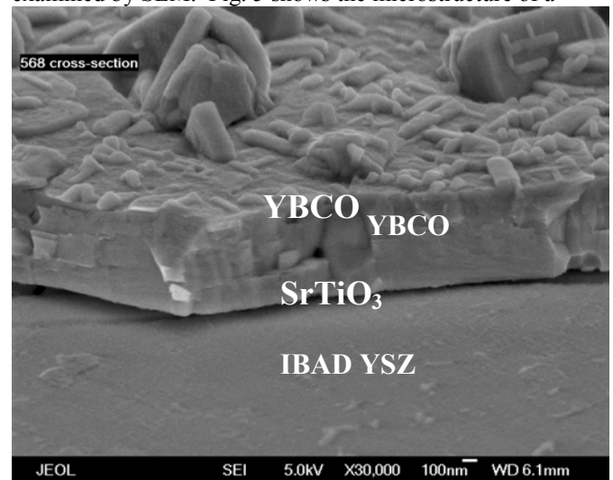
Fig. 5 Fracture surface of a YBCO film on an IBAD YSZ substrate. A dense film structure with abundant particles on surface is seen.
