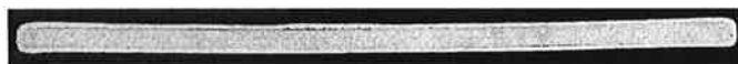
Fig. 5. Cross section of a coated conductor with surround copper stabilizer applied by electroplating.
