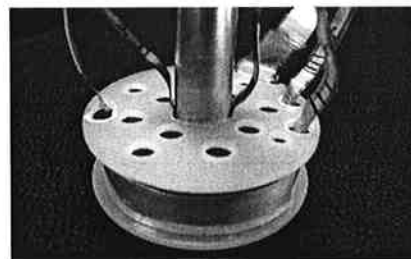
Fig. 10. Photograph of pancake coil fabricated with 7.4 m of coated conductor..
