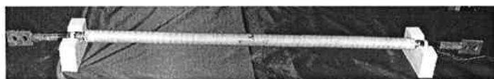
Fig. 8. Photograph of an 1 m long cable fabricated with 4 mm wide, copper stabilized coated conductor.
