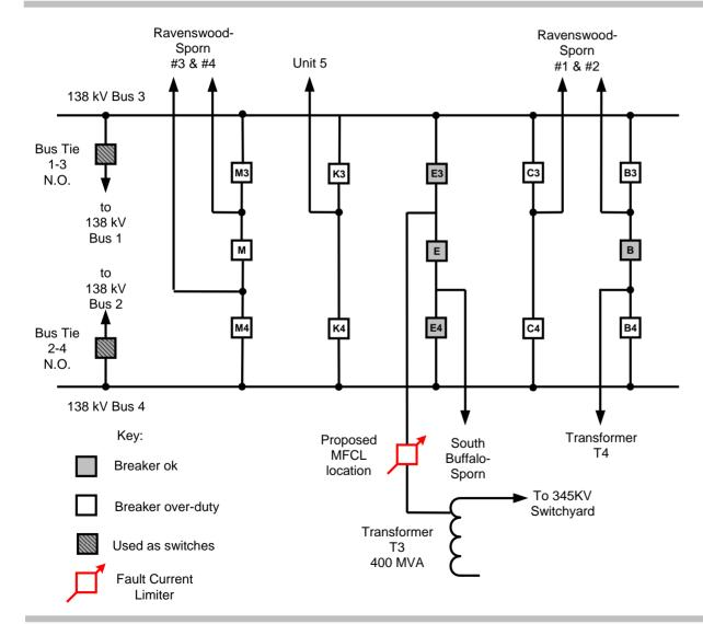
MFCL targeted to reduce fault contribution from transformer T3 when fault occurs in 138kV system
