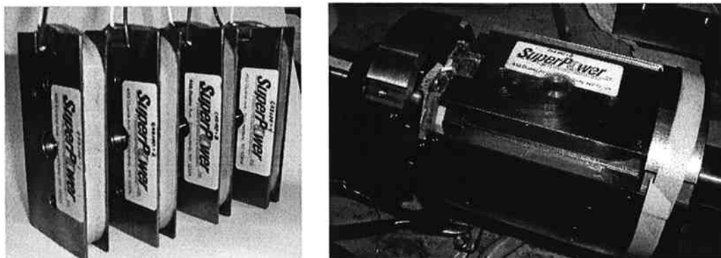
FIGURE 10 a) Four of the racetrack coils supplied to Rockwell Automation by SuperPower using 2G conductor. b) Racetrack coils mounted on the 3.7 kW (5 hp) rotor assembly.
