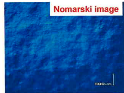
Electropolished tape – no grain boundaries
