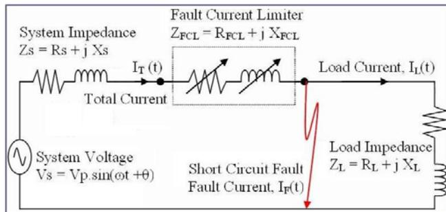
Fig. 1. Schematic diagram of single-phase power system representation.
