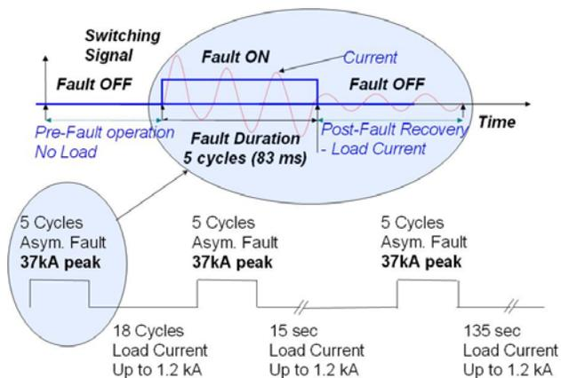
Fig. 2. AEP reclosure sequence for the first (3) faults.
