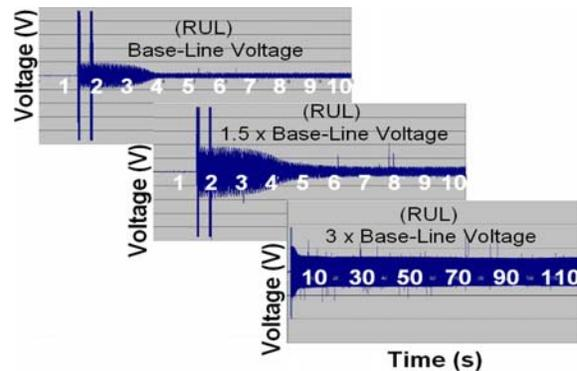
Fig. 6. Recovery under load for base-line voltage, 150% and 300%.
