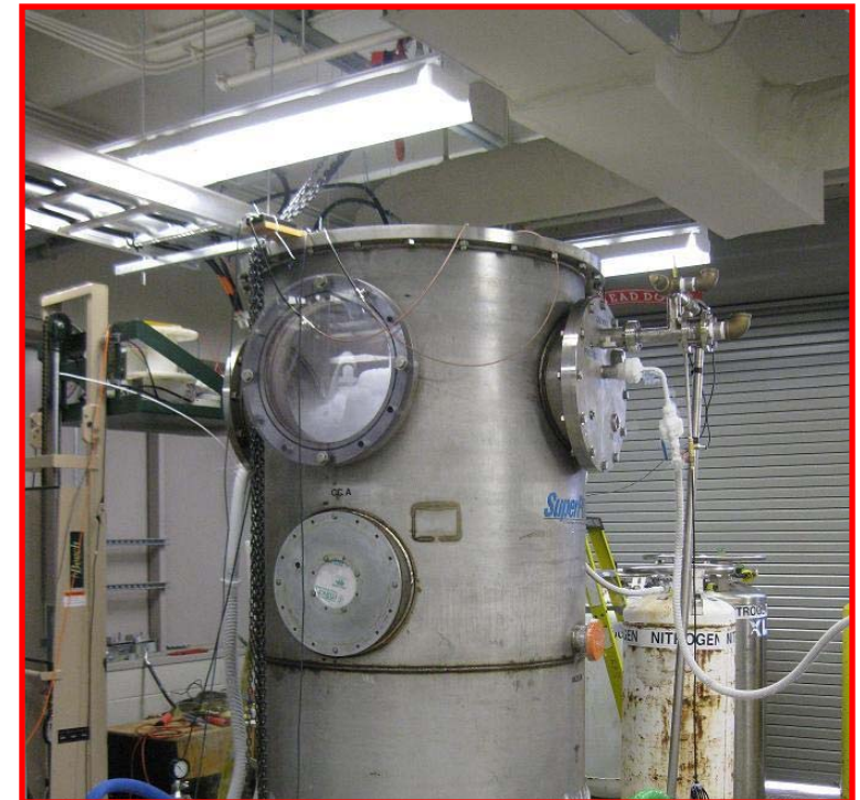
SFCL Device under test
