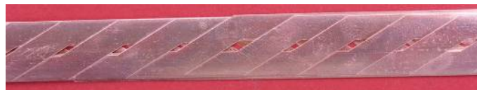
Fig. 6. A section of Roebel cable constructed by KIT using SP 2G HTS wire providing the transposition required for lowering the coupling loss component of the ac losses. Total width of the cable is 12 mm.
