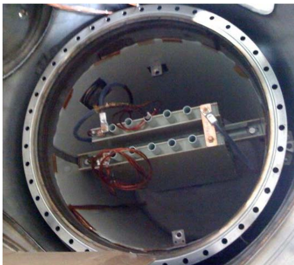
Fig. 8. View of a pair of 2G HTS based SFCL modules in a test cryostat. Operation is in LN 2 .
