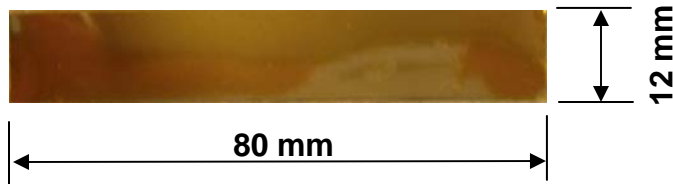
T-peel test on reference samples fabricated using Kapton adhesive tape/Hastelloy substrate
