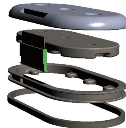
Superconducting Rotor Pole Design for fabrication & testing of coils with improved wire
