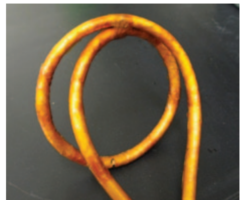
The cable that carried a world-record current of 4100 amperes in a background field of 19.81 T.
