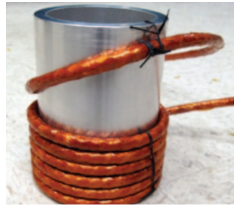
The six windings that form the inner layer of the magnet.
