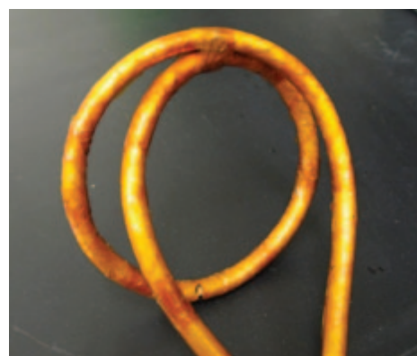
The cable that carried a world-record current of 4100 amperes in a background field of 19.81 T.
