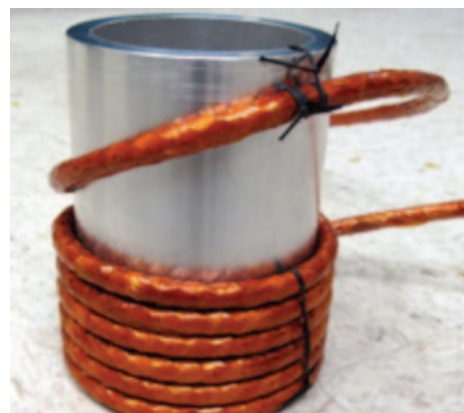
The six windings that form the inner layer of the magnet.
